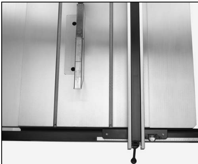
Figure 29. Aligning fence parallel to miter slot.
